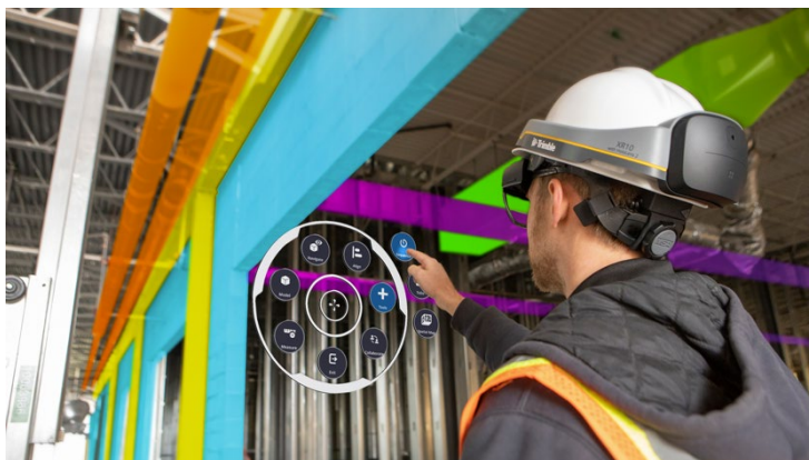
Field worker using Trimble’s XR10 with HoloLens 2, which uses mixed reality technology to take 3D content off the screen and into the real world to perform immersive pre-construction walk-throughs.
